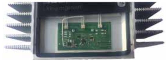
SES Lighting radio dimming transmitter
